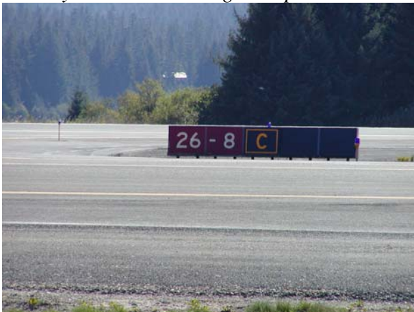
Runway Hold Position Sign sample
